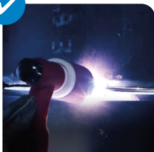
Wire feed in argon arc welding, observe molten pool in gap.
